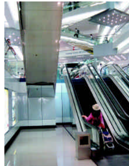
6.7.2e) Provide sufficient clearance between escalators
