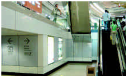
6.7.2b) Provide signage for an accessible route
