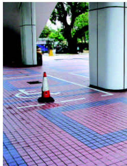
6.3.2b) Locate parking space for persons with a disability near building entrance and lift
