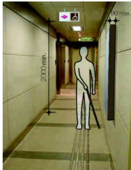
6.5.1b) Avoid protruding object along passageway
